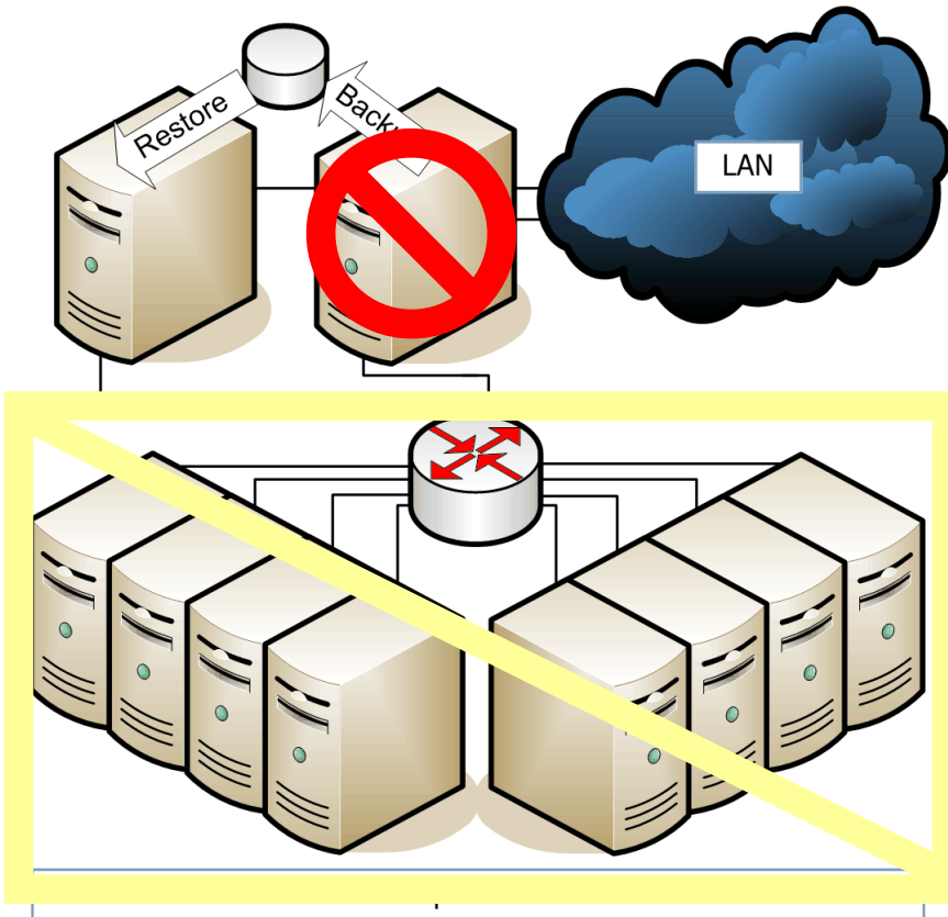
Active/Standby Head Nodes with Shared Storage
