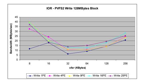
Fig. 4. PVFS2 Performance Tests: Write
