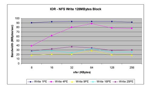
Fig. 2. NFSv4 Performance Tests: Write
